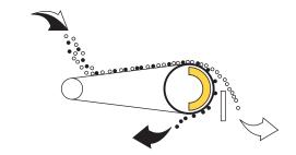
separation efficiency include Drum Speed, Splitter location, Magnet type and Pole configuration.
