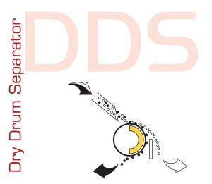
The main application of Dry Drum Magnet separator includes purification of raw materials in Glass, Tile, Ceramic, Food, Recycling, Casting and steel foundry industries, beside that it can be used widely for Iron ore Concentration or Ferro Alloy treatment. Apart from that conventional application this type of separator has found a wide range of other applications such as:
