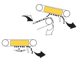
OVP magnets are used when substantial quantities of ferrous metals and or long and bulky pieces are contained in the conveyor burden or where access to the suspension magnet for cleaning is difficult. Iron contamination material is attracted by the magnet and is carry out of the magnetic field and ejected by the discharge belt running around the magnet.
