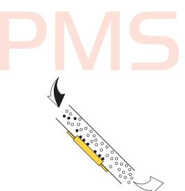
PMS Plate magnetic separator widely used for separation of tramp iron contamination through non-magnetic material to protection of valuable and worthy equipment in production processes against any damage and depreciation comes out interring the Ironic particles or unpurified materials in order to improved the output quality.
