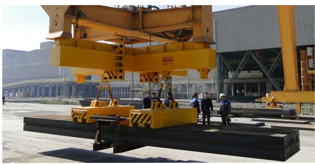
To increase the life time of magnet, the control panel equipped with a temperature and duty factor relays, and rectifier protected against any output short circuit accident. The accessory equipments include of battery backup device, cable reel, suspension chains and power supply socket.
